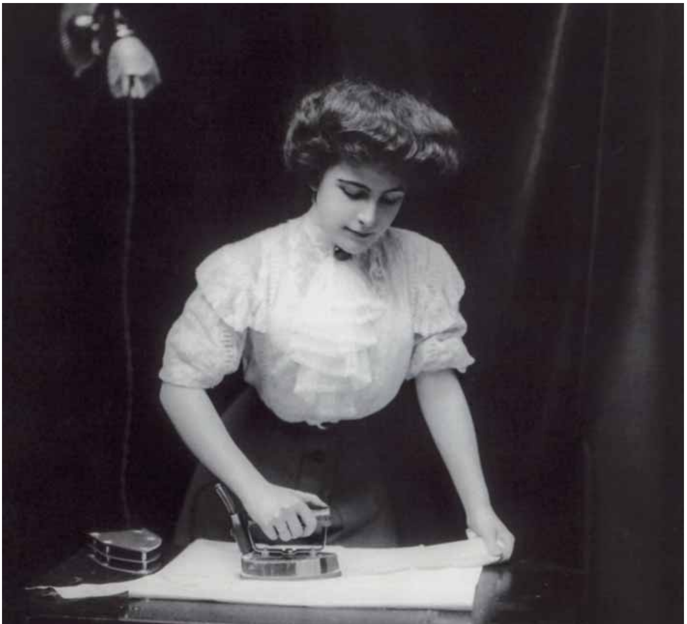
One of the first electrical appliances embraced by families was the electric iron, which plugged into a lightbulb outlet before wall plugs became standardized.
