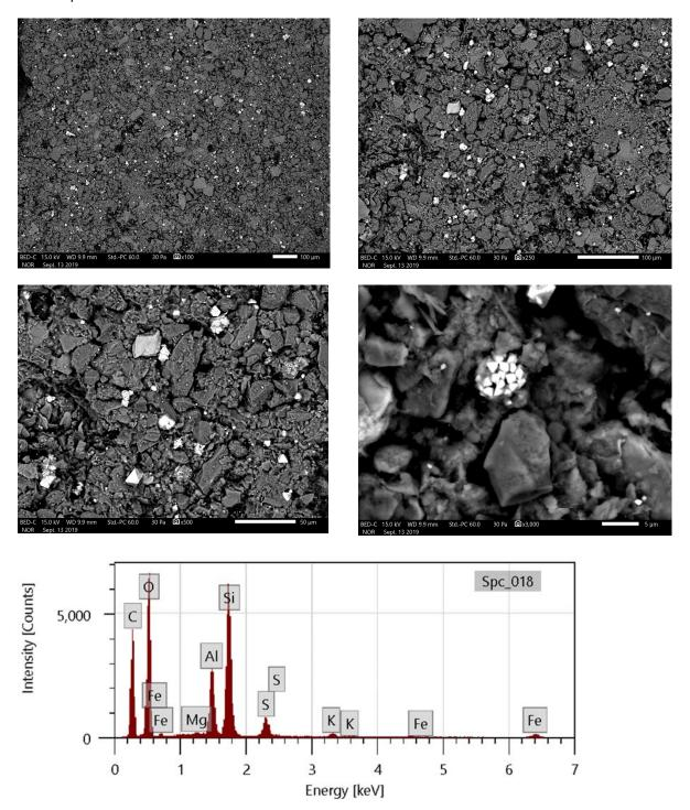
Sample VAP B3 40-45. Backscattered electron micrographs show the sample at 100X, 250X, 500X, and 3000X. EDS spectrum at bottom is an area scan of the region shown at 500X. Bright particles are pyrite (framboid in bottom right micrograph). Major peaks for carbon, oxygen, silicon, and aluminum suggest coal and clay.
