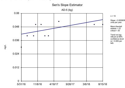
Constituent: Boron, total Analysis Run 12/16/2018 8:16 AM View: Trend Tests Welsh PBAP Client: Geosyntec Data: Welsh PBAP
