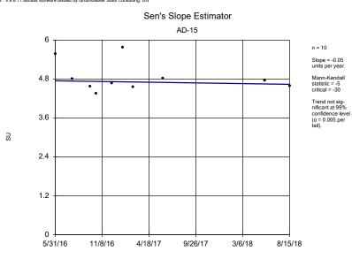
Constituent: pH, field Analysis Run 12/16/2018 8:16 AM View: Trend Tests Welsh PBAP Client: Geosyntec Data: Welsh PBAP
