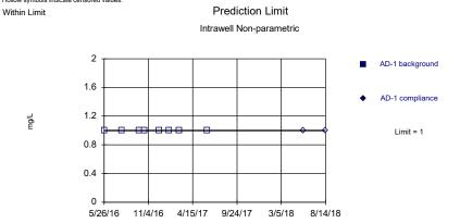
Non-parametric test used in lieu of parametric prediction limit because censored data exceeded 50%. All background values (n = 8) were censored; limit is most recent reporting limit. Well-constituent pair annual alpha = 0.04242. Individual comparison alpha = 0.02144 (1 of 2).
