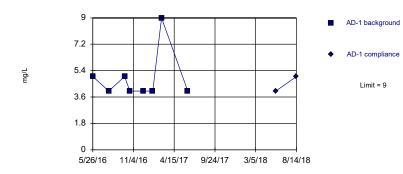
Non-parametric test used in lieu of parametric prediction limit because the Shapiro Wilk normality test showed the data to be non-normal at the 0.01 alpha level. Limit is highest of 8 background values. Well-constituent pair annual alpha = 0.04242. Individual comparison alpha = 0.02144 (1 of 2).
