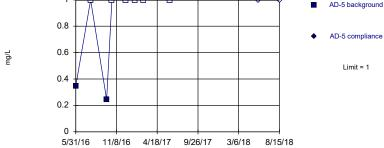
Non-parametric test used in lieu of parametric prediction limit because censored data exceeded 50%. Limit is highest of 8 background values. 75% NDs. Well-constituent pair annual alpha = 0.04242. Individual comparison alpha = 0.02144 (1 of 2).
