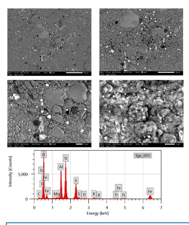
Sample VAP B3 50-55. Backscattered electron micrographs show the sample at 250X, 500X, 1000X, and 3000X. EDS spectrum at bottom is an area scan of the region shown at 3000X. Bright particles are mostly pyrite (framboid in bottom left micrograph); occasional particles of Fe-Ti oxide are detected. Major peaks for oxygen, silicon, and aluminum suggest clay. Large blocky particles are mostly quartz, feldspar, and clay.
