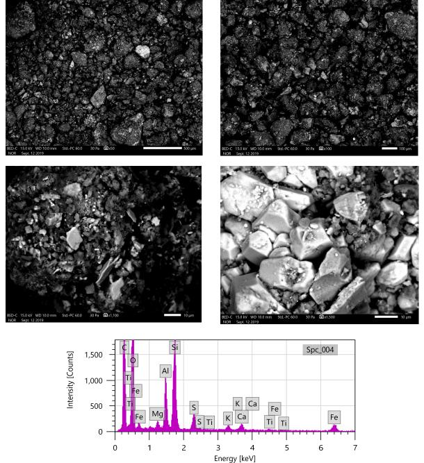
Lignite. Backscattered electron micrographs show the sample at 100X, 1,100X, and 1,500X. EDS spectrum at bottom is an area scan of the region shown in top right micrograph. Bright particles are mostly quartz and feldspar. Major peaks for carbon, oxygen, silicon, and aluminum suggest coal and clay.
