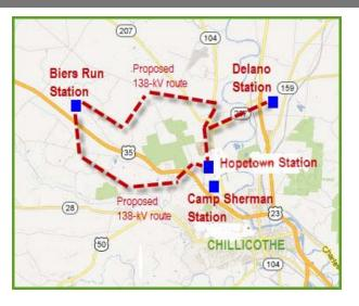
b1032.2 - Construct two 138kV outlets to Delano 138kV station and Circleville station; install new 138 kV breaker string at Delano station to terminate new line.
