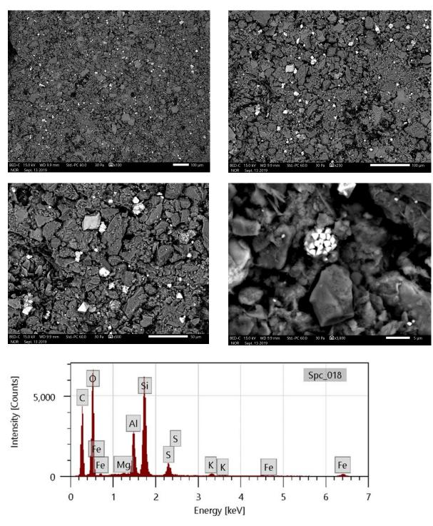
Sample VAP B3 40-45. Backscattered electron micrographs show the sample at 100X, 250X, 500X, and 3000X. EDS spectrum at bottom is an area scan of the region shown at 500X. Bright particles are pyrite (framboid in bottom right micrograph). Major peaks for carbon, oxygen, silicon, and aluminum suggest coal and clay.
