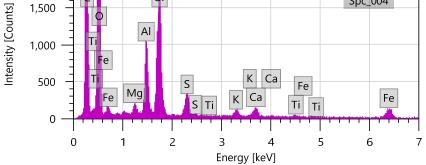
Lignite. Backscattered electron micrographs show the sample at 100X, 1,100X, and 1,500X. EDS spectrum at bottom is an area scan of the region shown in top right micrograph. Bright particles are mostly quartz and feldspar. Major peaks for carbon, oxygen, silicon, and aluminum suggest coal and clay.
