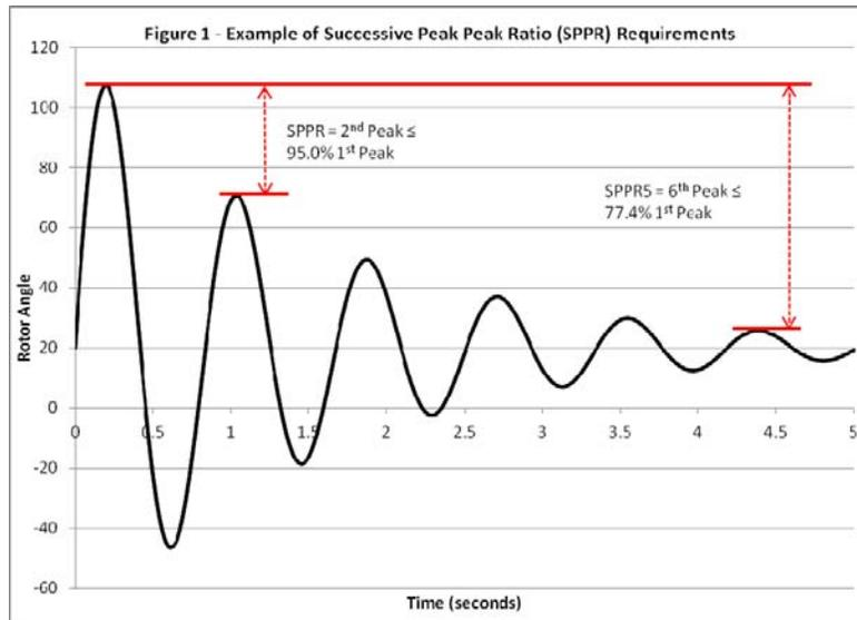
Figure 2: Example of Successive Positive Peak Ratio (SPPR) Requirements
