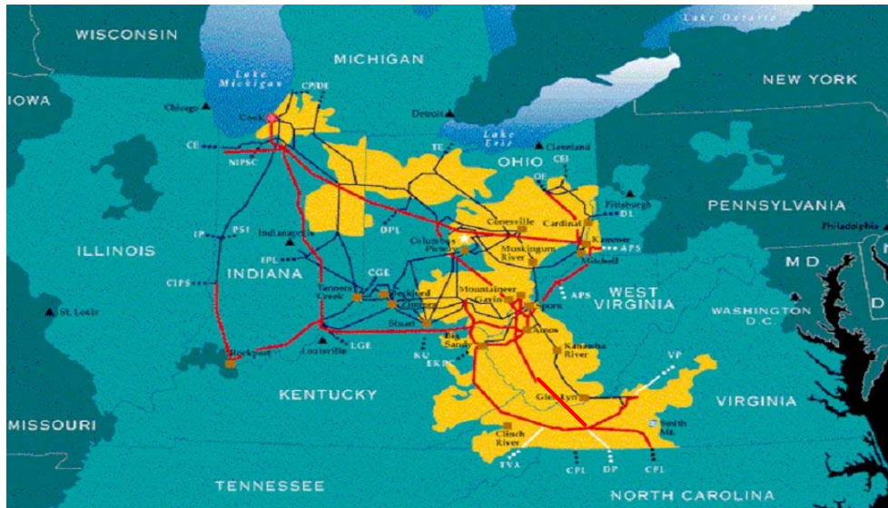
Figure 1. AEP Eastern Transmission, Including 765-kV (Red) and 345-kV (Blue) Lines
