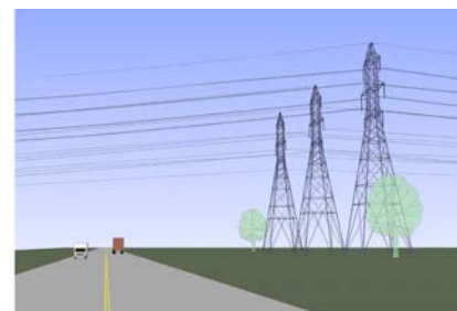
345 kV Three Double Circuit Towers (450 ft. Right-of-Way)
