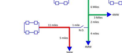
MW-mile = 4 MW\*(6 miles + 3 miles) + 4 MW\*(6 miles + 2 miles + 4 miles) = 84 MW-mile MW-mile = 3 MW\*(11 miles + 5 miles) = 48 MW-mile
