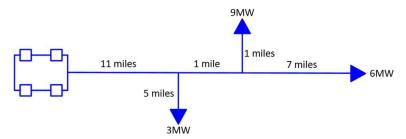
MW-mile = 3 MW\*(5 miles + 11 miles) + 9 MW\*(11 miles + 1 mile + 1 mile) + 6 MW\*(11 miles + 1 mile + 7 miles) = 279 MW-mile
