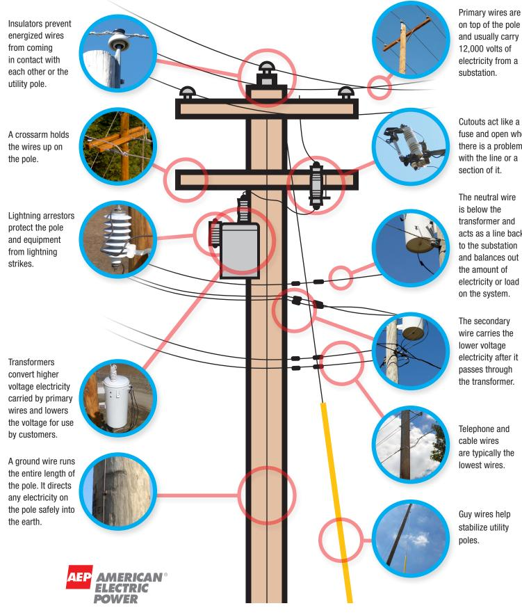
on top of the pole and usually carry electricity from a
